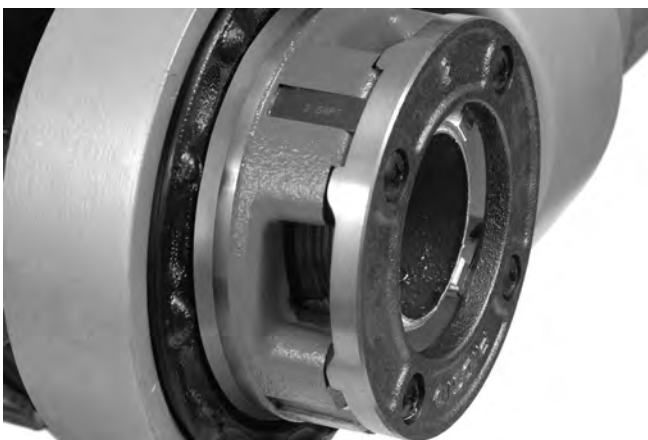
Figure 15 – Pipe Even with Edge of Dies
