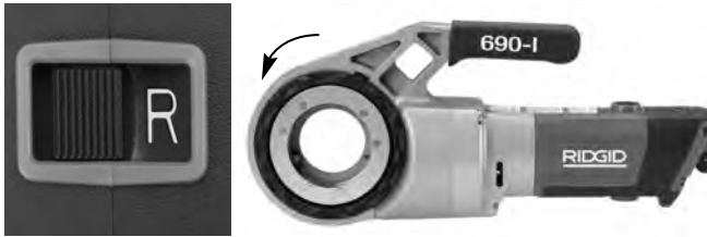
Figure 6B – R (REVERSE) (Counter-Clockwise) Switch Position
