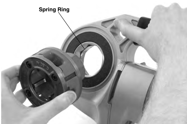
Figure 9 – Installing Die Heads into 600-I Power Drive
