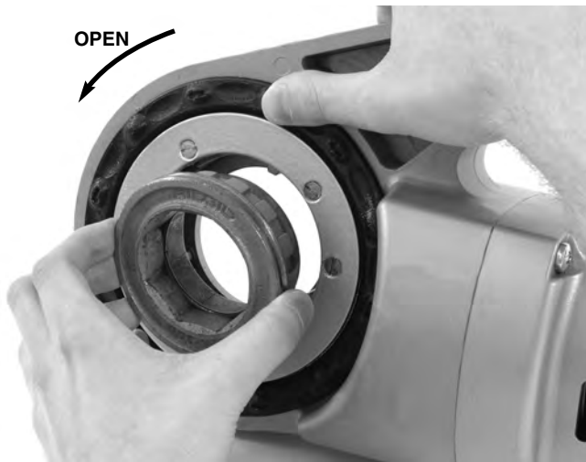
Figure 8 – Installing Adapter Into 690-I
