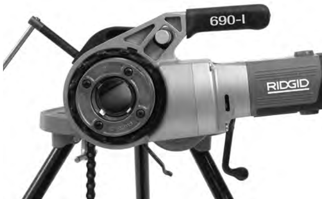
Figure 12 – Proper Orientation of the Power Drive
