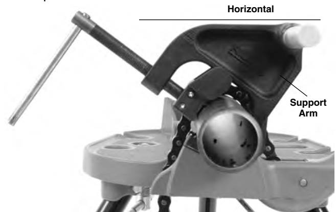
Figure 11A – Positioning the Support Arm
